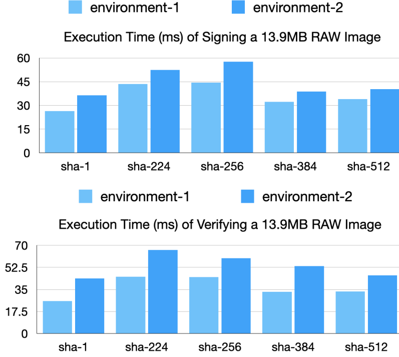
Figure 8: Execution time of signing and verifying a high-quality lossless format image.
